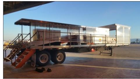
One of the company's recent adaptation's, shown above, is two Adjustoveyors mounted on a flatbed trailer that is used by FedEx to load and unload trucks at its major airport hubs around the world.
